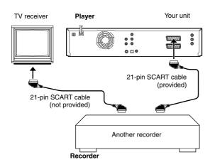
2 When using your unit as the recording deck:
